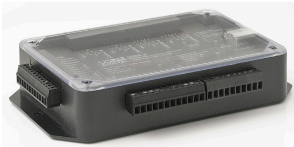
Figure 2: Mr. Linden's current connector, a USB4 from US Digital. Showing manually wired plugins
